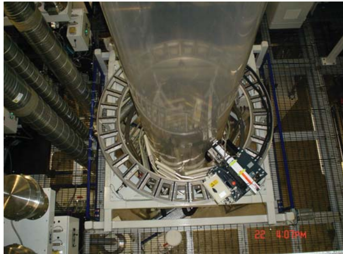
Co-extruder produces high quality films with consistent gauge thickness.
